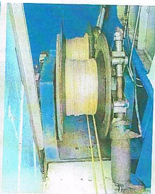
STRENGTH: The 10mm Dyneema rope used to replace Katrine Kim's conventional steel wire rope warps
