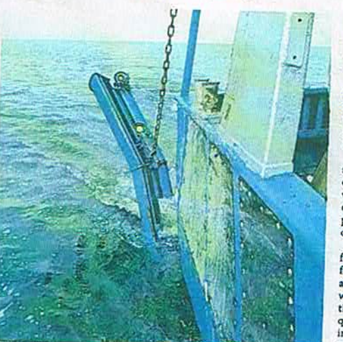
SWITCH: One of the 2m 2 Thyborøn Type 15 doors on the surface. These were replaced during the project with a 1.50m 2 pair
