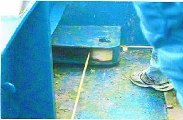
Nylonrollers for protection against wear
