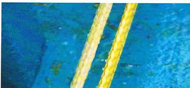
The Dyneema rope after one years service
