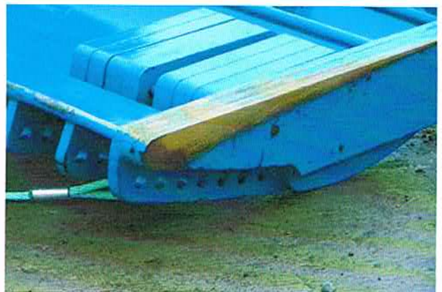
The trawl door after one year of service
